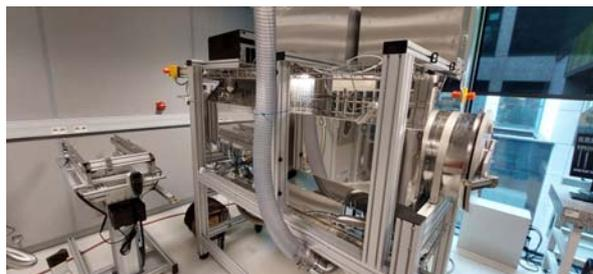
Fig. 4. ALD reactor BENEQ P400, used for the deposition of thin transparent electrodes.
