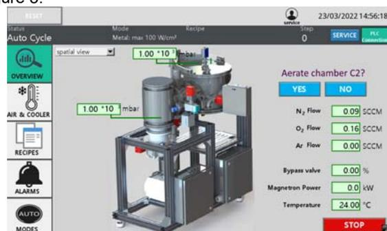
Fig. 2. System operator desktop (PVD) with fields for entering process data.
