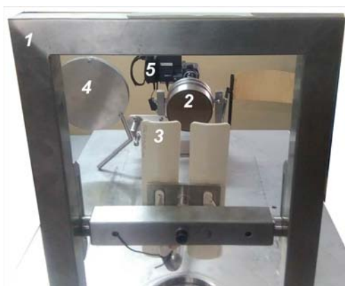
Fig. 4. Diagram of the test stand for testing the effect of thermal radiation on material samples. 1 - support frame, 2 - test material, 3 – radiator, 4 – shutter, 5 - thermal imaging camera
