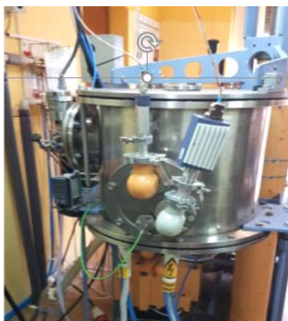
Fig. 1. Vacuum equipment for protective film deposition
