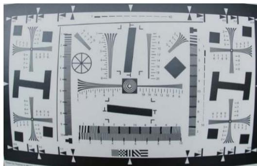
C. Image from Camera IMX477 with 6 mm CS-Mount lens
