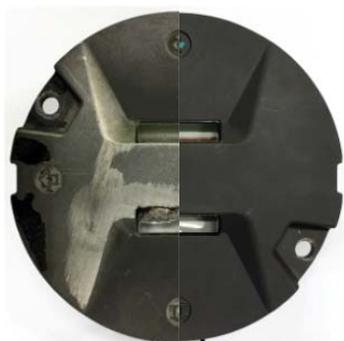
Fig.1. Runway center line lamp - damaged (left) and new (right)
