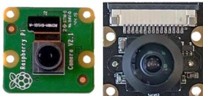
Fig.9. Raspberry Pi Camera HD v2 with a viewing angle of 62.2° (a) and Waveshare 16579 160° (b)
