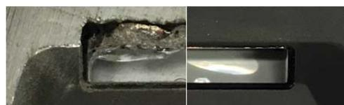
Fig.2. Runway centerline lamp prism - damaged (left) and new (right)
