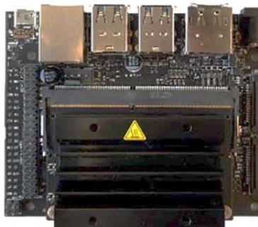
Fig.7. Nvidia Jetson Nano 4GB microcomputer
