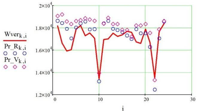
Fig.6. Comparison of forecast and actual values for the recurrent neural network and the vector method, where the solid line is actual data, dots are the forecast values of the recurrent neural network, and the diamonds are the forecast values of the vector method. The abscissa is hours, and the ordinate is electricity consumption, kW\*h.
