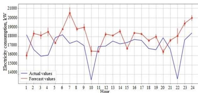
Fig.5. Comparison of actual and forecast values by the wavelet transform
