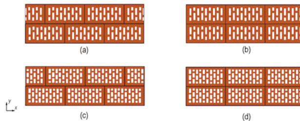
Fig.3. The four kinds of analysed wall: a) asymmetric composed of B18 bricks (B18\_asym); b) symmetric composed of B18 bricks (B18\_sym); c) asymmetric composed of B30 bricks (B30\_asym); d) symmetric composed of B30 bricks (B30\_sym)
