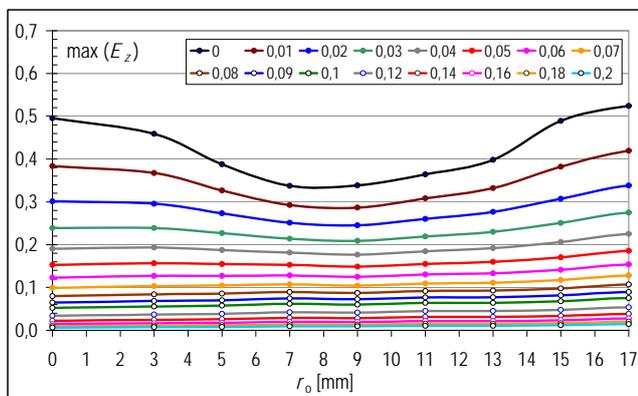
Fig.4. The relative maximum values of  $E_z$  component behind the wall made of B18 bricks (model asymmetric – B18\_asy)
