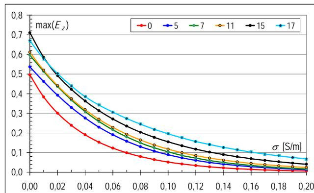
Fig.11. The relationship between conductivity and the size of hollow in the model B30\_sym
