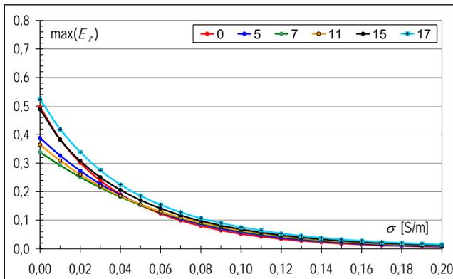
Fig.8. The relationship between conductivity and the size of hollow in the model B18\_asym
