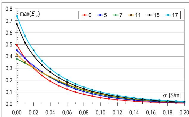
Fig.9. The relationship between conductivity and the size of hollow in the model B18\_sym
