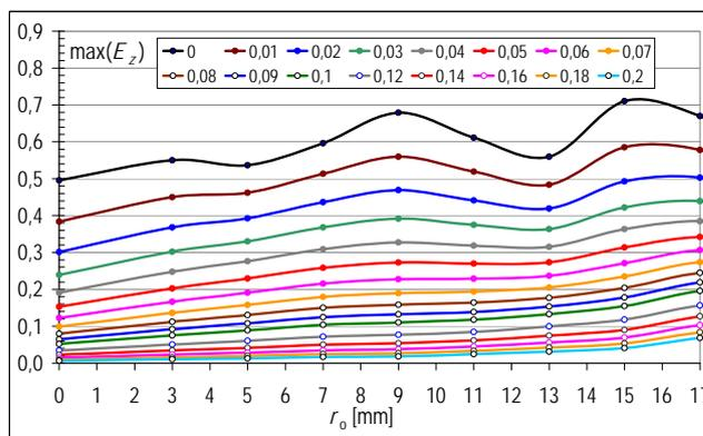
Fig.7. The relative  $\max(E_z)$  component behind the wall made of B30 bricks (model symmetric – B30\_sym)
