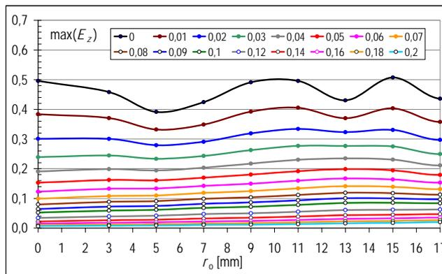
Fig.6. The relative maximum values of  $E_z$  component behind the wall made of B30 bricks (model asymmetric – B30\_asy)
