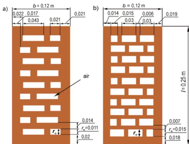
Fig.2. Geometrical sizes of two types of analysed brick: a) B18 and b) B30
