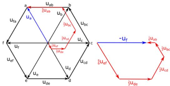
Figure 2. The dependencies between voltages vectors  $U_a, -U_f$  and phase-to-phase voltage vectors.
