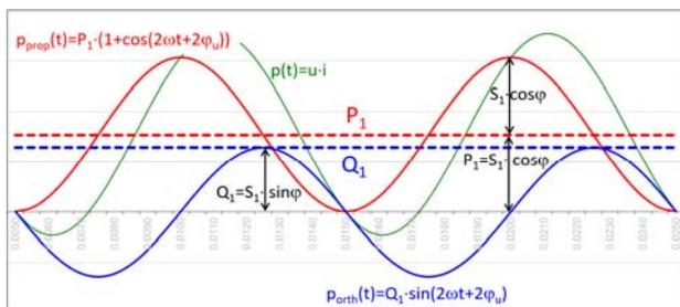
Fig. 2. Power oscillations, sinusoidal case
