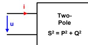
Fig. 1. Electric two-pole (single-phase system) with periodical voltage and current
