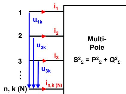
Fig. 5. Electric n-pole in general
