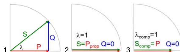
Fig. 3. Power orthogonality relation: 1 general, 2 equiv. proportional case, 3 compensated case
