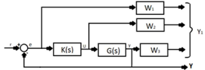
Fig.1. The augmented plane
