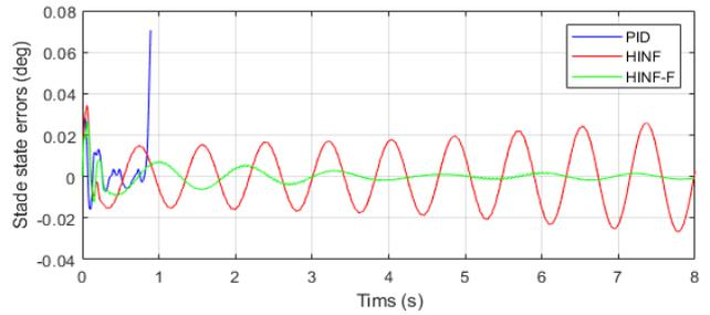
Fig. 17. The state state error for joint 1 ( $\mathcal{G}_1$ )
