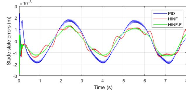
Fig.11.The stade state error for Y-axes
