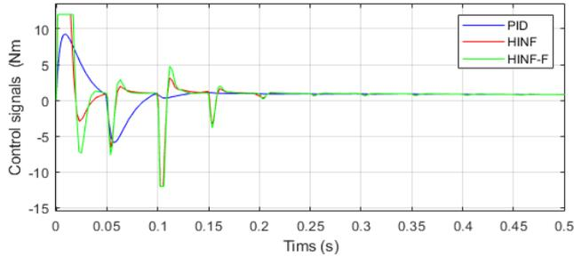
Fig. 15. The control signals for joint 3 ( $\mathcal{G}_3$ )
