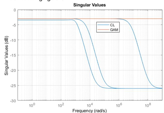
Fig.5. singular values of the Closed-Loop for Hinf control
