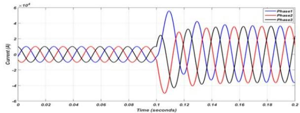
Fig. 9. Primary current external fault
