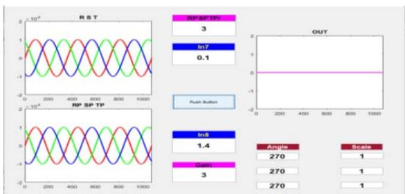
Fig. 13. Primary and secondary currents at no fault
