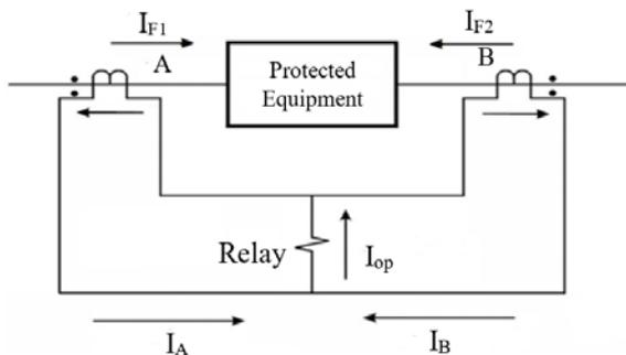
Fig.2. A single-line diagram of a differential relay fault that is zone.
