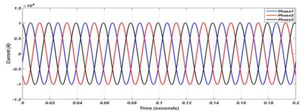
Fig. 8. Primary current without fault.
