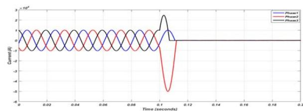
Fig.11. Line-Line to ground (L-L-G) fault
