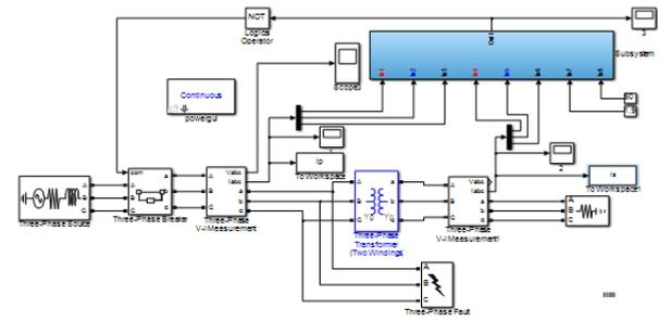
Fig.7. Complete circuit of power system.
