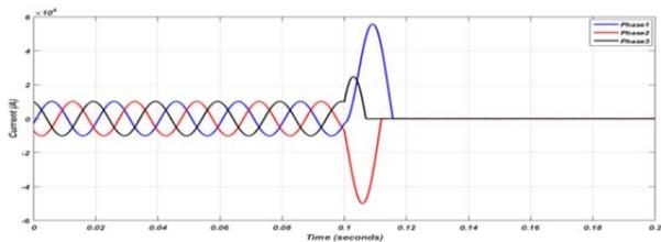
Fig. 12. Three phase to ground fault
