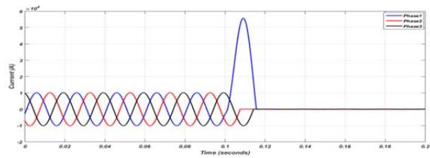
Fig. 10. Line to ground (L-G) fault
