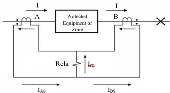
Fig.1. A single-line diagram of a differential relay fault that is out of zone.
