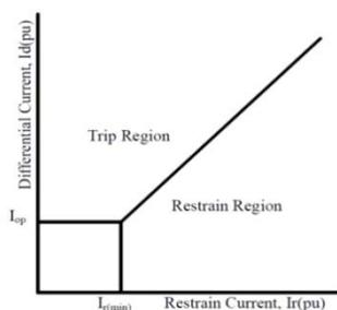
Fig.3. Differential relay characteristics.
