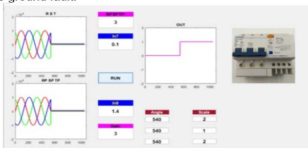
Fig. 16. Current at line to line to ground (L-L-G) fault
