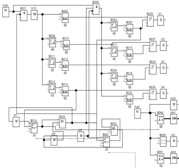
Fig. 3. Control program for the stepper motors using One-phase ON stepping excitation method
