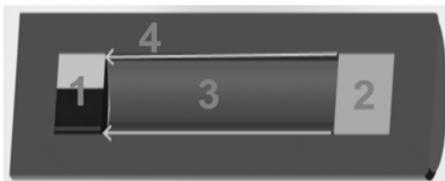
Fig. 2. Typical regions of heat pipes. 1 - boiling and evaporation region; 2 - liquefaction region; 3 - gas phase; 4 - return of liquid phase
