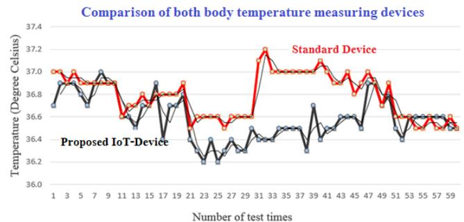
Fig. 4 The calibration test between the proposed IoT device and the standard one
