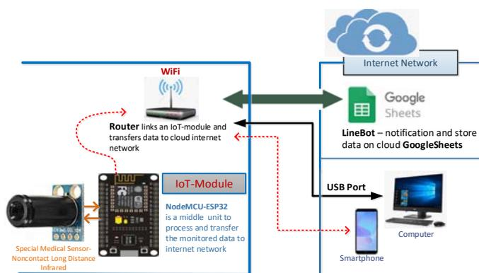
Fig.1 The architecture of the proposed RPBTM framework
