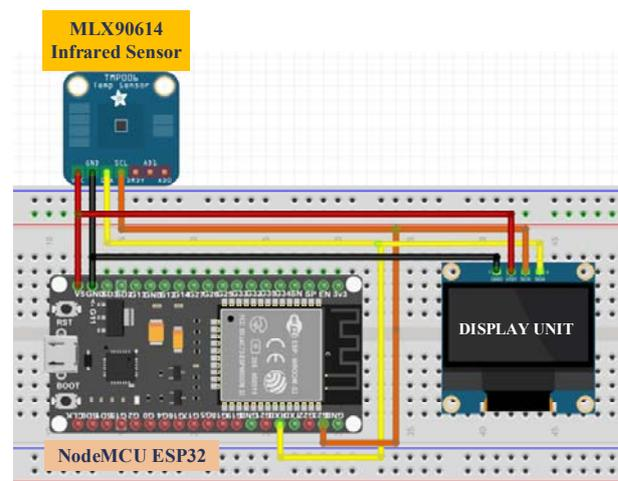
Fig.2 Schematic circuit of the hardware device
