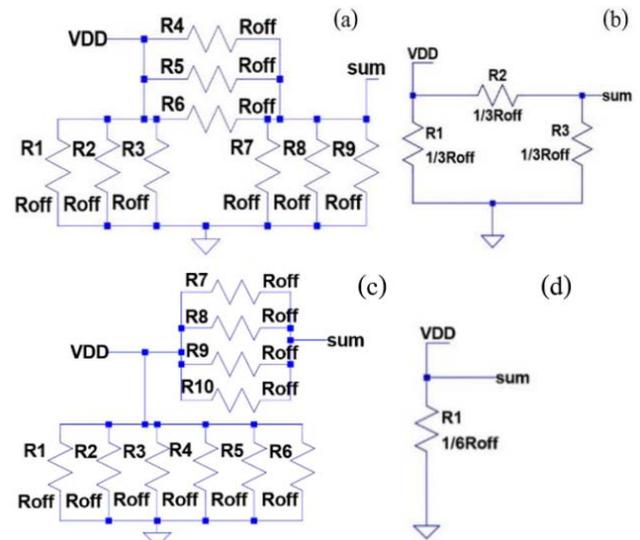
Fig. 8 The equivalent circuit of the multi-input MRL 1-bit full adder: (a) even number of HIGH, (b) simplified equivalent circuit given even number of HIGH, (c) odd number of HIGH, (d) simplified equivalent circuit odd number of HIGH
