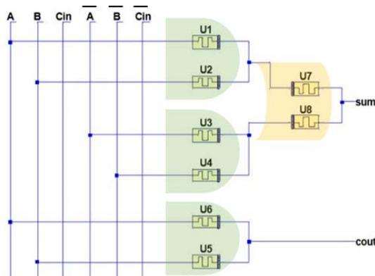
Fig. 2 Multi-stage memristor-based half adder circuit
