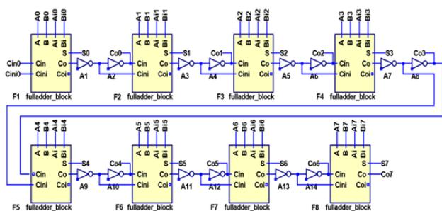
Fig. 9 The proposed multi-input MRL 8-bit full adder circuit consisting of eight blocks of 1-bit full adders with CMOS inverters
