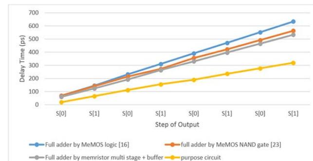
Fig .11 Simulated delay time of multi-input MRL 8-bit full adder circuit as a function of incremental adder blocks
