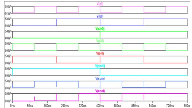
Fig. 10 Simulated voltage output (sum and carry out) of multi-input MRL 1-bit full adder circuit given six voltage inputs
