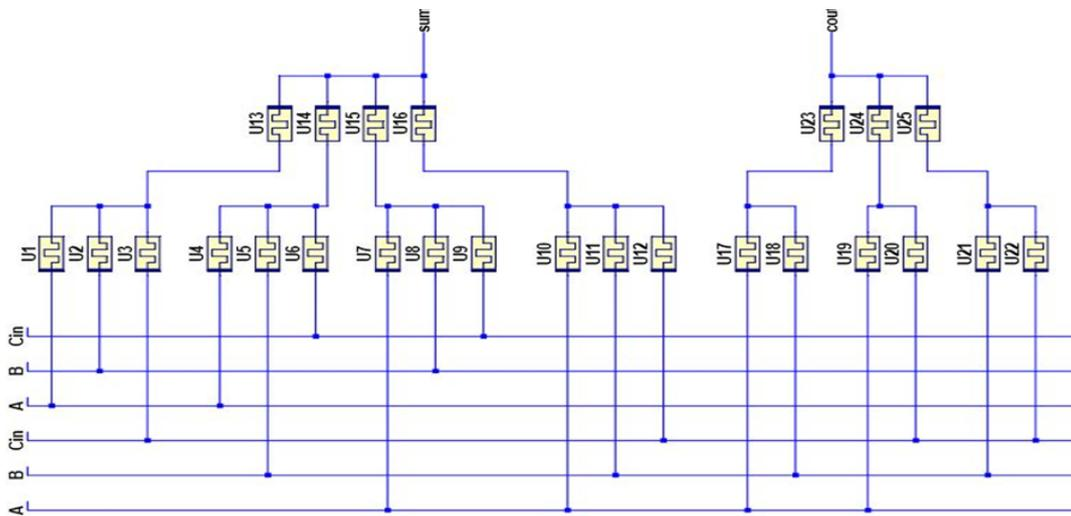
Fig. 7 The proposed multi-input MRL 1-bit full adder circuit consisting of 25 memristors
