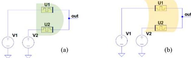
Fig. 1 Two-input MRL gates: (a) AND gate, (2) OR gate [9]
