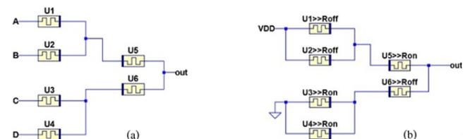
Fig. 4 Multi-stage memristor-based circuits: (a) two-stage AND/OR logic circuit, (b) two-stage logic circuit functioning
