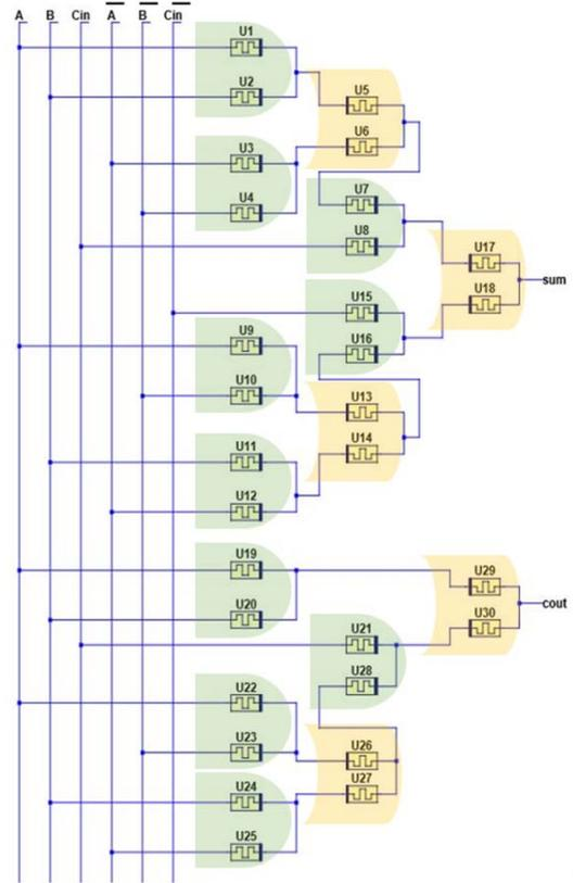
Fig. 3 Multi-stage memristor-based full adder circuit
