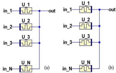
Fig. 5 The proposed multi-input MRL gates: (a) multi-input AND gate, (b) multi-input OR gate
