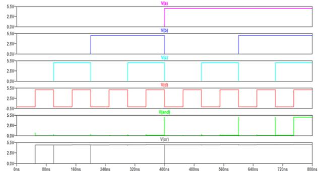
Fig. 6 Simulated voltage outputs of multi-input MRL AND and OR gates, given four voltage inputs
