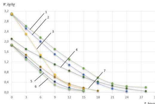
Fig. 3. Drying kinetics from proportion air flow  $G_n$  ( $\text{m}^3 / \text{h}$ ) at  $P_{sh} = 44.2 \text{ kg / m}^2$ ;  $\Delta d = 10 \text{ gr.moist / kg.sp.}$ : 1 – 500; 2 – 560; 3 – 1115; 4 – 340; 5 – 875; 6 – 910; 7 – 480.
