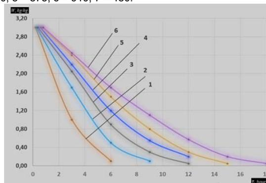
Fig. 4. Kinetics of drying from the proportion of specific load of the material  $P_{sh}$  ( $\text{kg / m}^2$ ) at  $\Delta d = 10,1 \text{ gr.moist./kg.sp.}$ ,  $G_n = 500 \text{ m}^3 / \text{h}$ : 1 – 13.8; 2 – 21.6; 3 – 28.9; 4 – 36.1; 5 – 43.5; 6 – 50.5.
