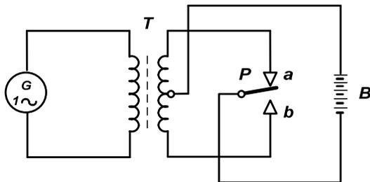
Fig.3. Basic elements and principle of operation of a mechanical rectifier: *G* - supplying alternating voltage source; *T* - transformer with tap in the secondary winding; *P* - mechanical switch; *B* - charged electrochemical battery
