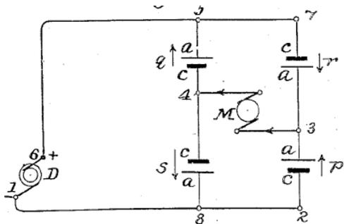
Fig. 5. The bridge circuit of a 1-phase electrolytic rectifier, included in the description of the American patent obtained by Charles Pollak [15]: D - alternating voltage source; M - receiver powered by rectified voltage; p, q, r, s - the cells of the electrolytic rectifier (marked with the symbols used for electrochemical cells)
