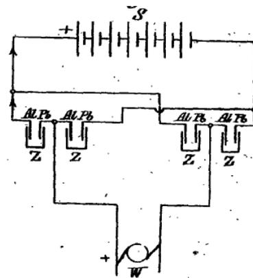
Fig.4. The bridge circuit of a 1-phase electrolytic rectifier included in the British patent specification obtained by Charles Pollak [13]: *W* - alternating voltage source; *Z* - electrolytic cell with Al and Pb electrodes; *S* - accumulator battery
