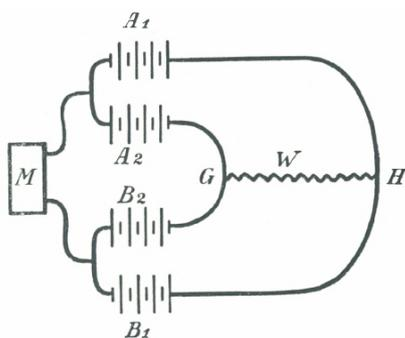
Fig.6. Bridge circuit of a 1-phase electrolytic rectifier developed by prof. Leo Graetz [16]: M - alternating voltage source; W - receiver powered by rectified voltage; A1, A2, B1, B2 - electrolytic rectifier cells
