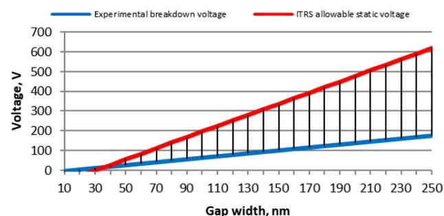
Fig 6. Breakdown voltage of experimental versus ITRS of Binary reticle
