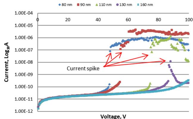
Fig.4. The IV curve of direct discharge test on Binary reticle feature with gap distance of 80, 90, 110, 130 and 160 nm
