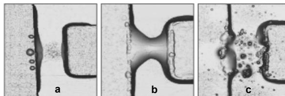
Fig.1. The transformation of reticle feature from the effect of EFM. A metal continuous diffuse (a) to adjacent metal until complete bridging (b) and end up vaporised (c) [14]
