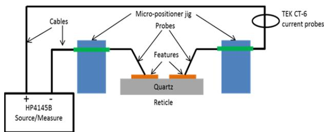
Fig.3. The schematic representation of electrostatic direct discharge test
