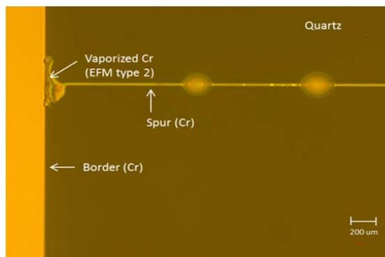
Fig 8. The 80 nm feature with EFM damage after direct discharge test
