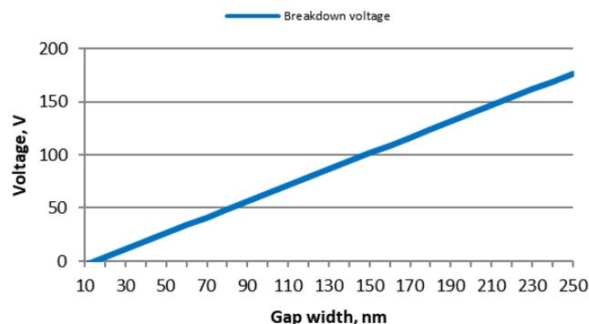
Fig 5. Breakdown voltage of nanometre scale gaps based on extrapolated data of 80 to 130 nm experimental quantification result
