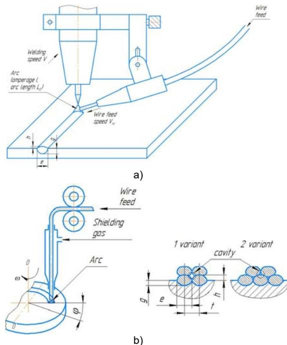
Fig. 2. The scheme of formation of the surfacing roller (a) and the process of reproduction of the model in the study and options for teaching the roller (b)
