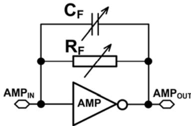
Fig.4. Inverter-based analog front-end
