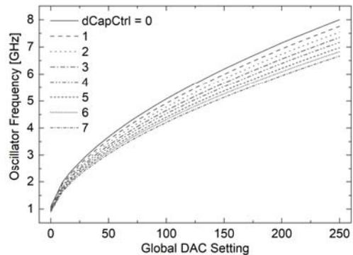
Fig.7. Post-layout ring oscillator simulation result: output frequency as a function of global 8-bit DAC word for all 8 possible settings of capacitance bank (dCapCtrl)
