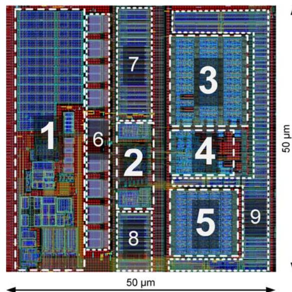
Fig.3. Pixel layout: 1 – analog front-end and references, 2 – oscillators and trimming DACs, 3 – counters/shift registers, 4 – logic and coincidence circuit, 5 – configuration register, 6-9 – decoupling capacitors
