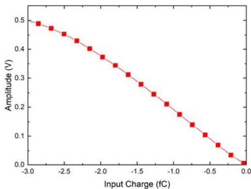
Fig.6. Front-end amplifier's linearity
