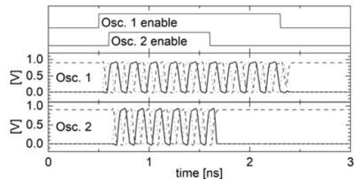
Fig.8. Exemplary transient post-layout simulation of the middle part of the pixel (oscillators with calibration blocks): oscillator enable inputs and three output phases per oscillator are visible
