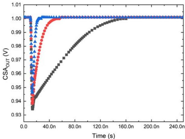
Fig.5. Front-end amplifier's output response for different feedback settings
