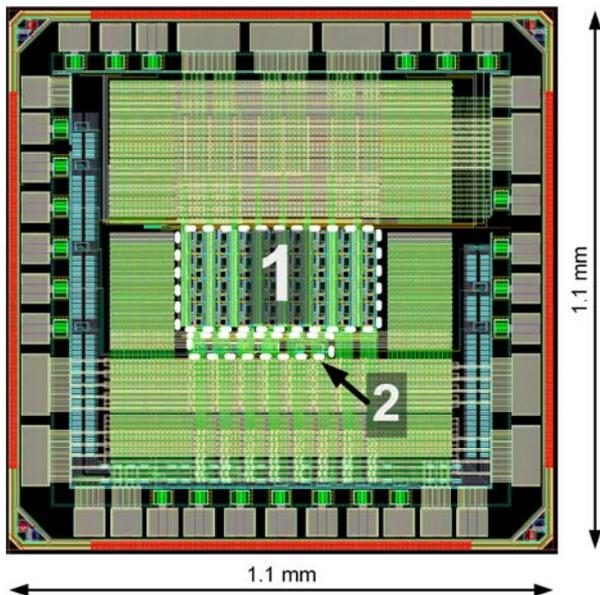
Fig.2. Chip layout: 1 – 8x4-pixel matrix, 2 – global part
