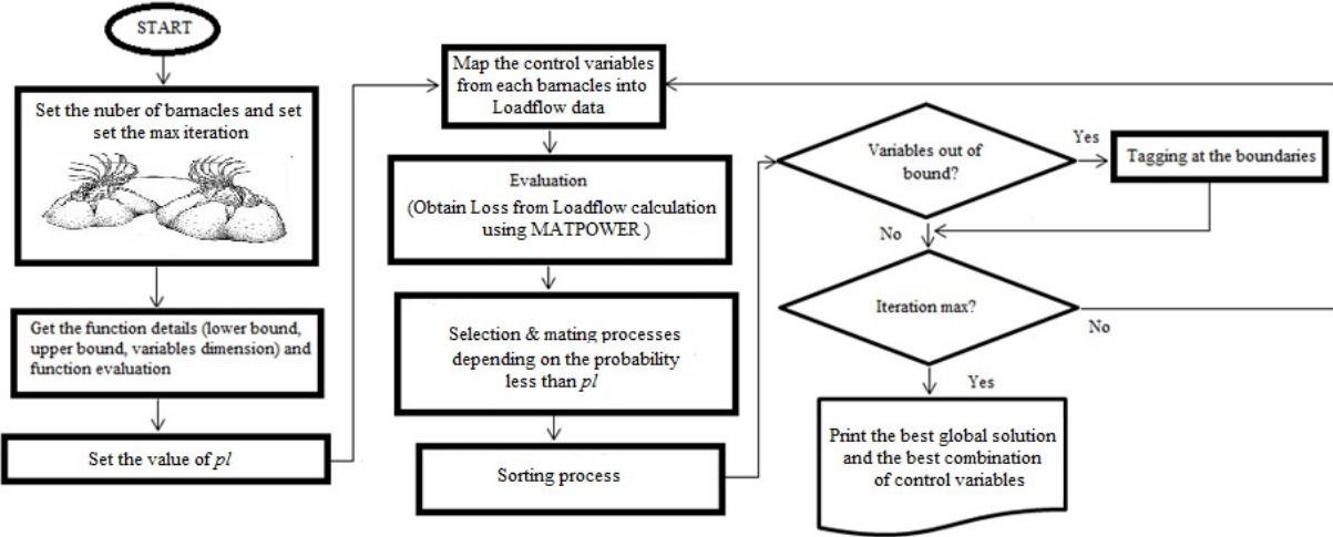
Fig.2. The flow of BMO to obtain minimum loss of ORPD
