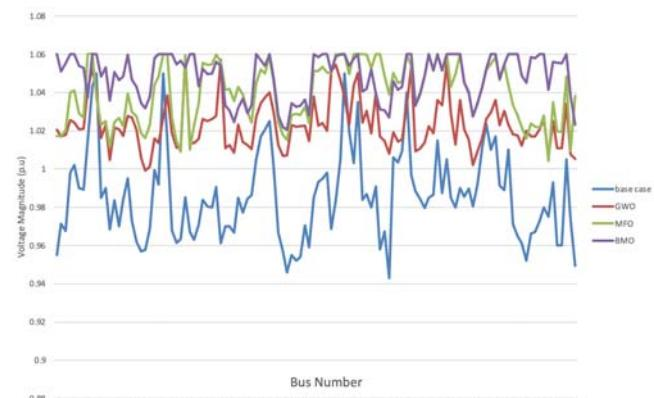
Fig.7. Voltage profiles for IEEE-118 bus system for base case, GWO, MFO and BMO
