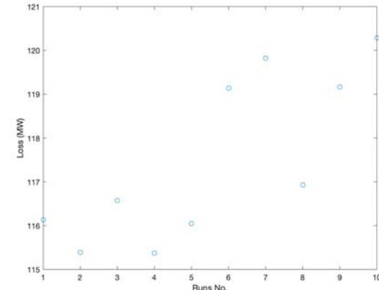
Fig.6. Performance for 30 barnacles for 10 free running of simulations of IEEE-118 bus system
