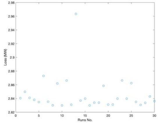
Fig.4. Results of the best objective (loss minimization) obtained by BMO for 30 simulations of 25 variables of IEEE-30 bus system
