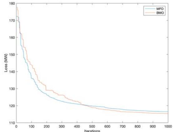
Fig.5. Convergence graph for the best results obtained by MFO vs BMO for IEEE-118 bus system
