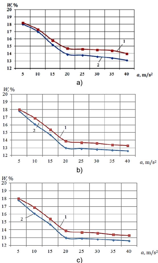
Fig. 4. The dependence of the change in the moisture content of grain raw materials depending on the vibration acceleration: a – at drying agent temperature  $45^\circ\text{C}$ ; b – at drying agent temperature  $55^\circ\text{C}$ ; c – at drying agent temperature  $65^\circ\text{C}$ ; 1 – at the technological loading of the drying chamber 75% from total volume; 2 – at the technological loading of the drying chamber 50% from total volume.
