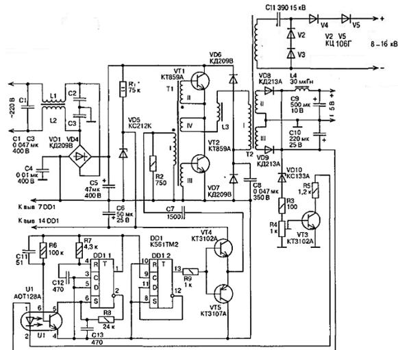
Fig. 3. Electrical circuit diagram of the power supply unit of the ozonizer based on a quasi-resonant converter.
