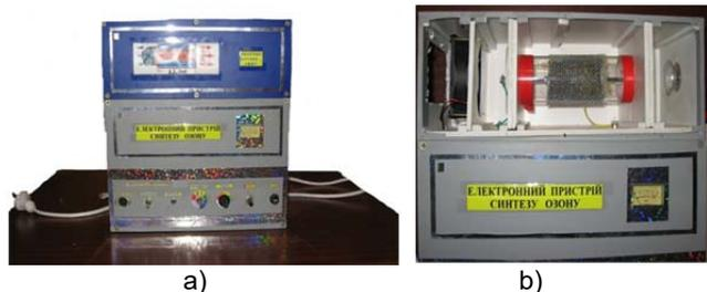
Fig. 2. Electronic ozone synthesis device: a – general form; b – ozone synthesis working chamber.
