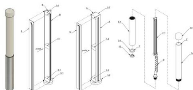
Fig. 6. Construction of a measuring probe shaped as a regular triangular prism and a regular rectangular prism
