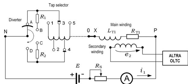
Fig. 2. Schematic diagram of the measurement method
