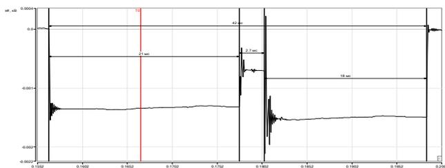
Fig.7. An example of a voltage curve recorded by the device during field testing of the OLTC
