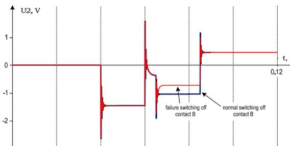
Fig.5. Voltage curve on transformer secondary winding under arcing switching-off contact B
