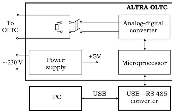
Fig.5. The layout of the proposed DRM setup
