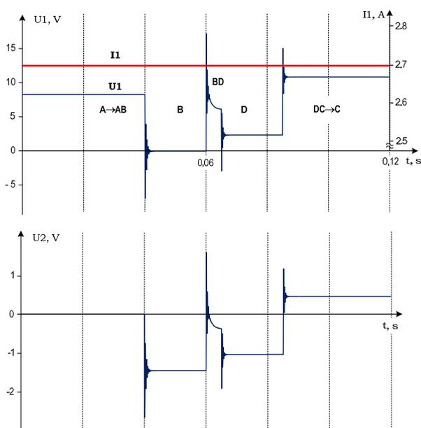
Fig.4. Primary voltage (U1) and current (I1) and secondary voltage (U2) curves under no-load secondary winding
