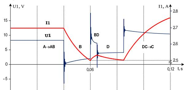
Fig.3. Primary voltage (U1) and current (I1) curves under shorted transformer secondary winding
