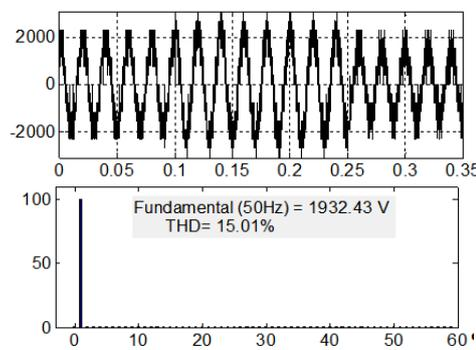
Figure 6.a) Inverter output voltage [volts], b) Harmonic content from the first phase of the compensator
