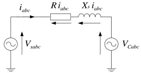
Figure 3. Equivalent circuit of the STATCOM.
