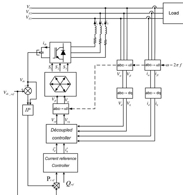
Fig. 4. Block diagram of the proposed control strategy.
