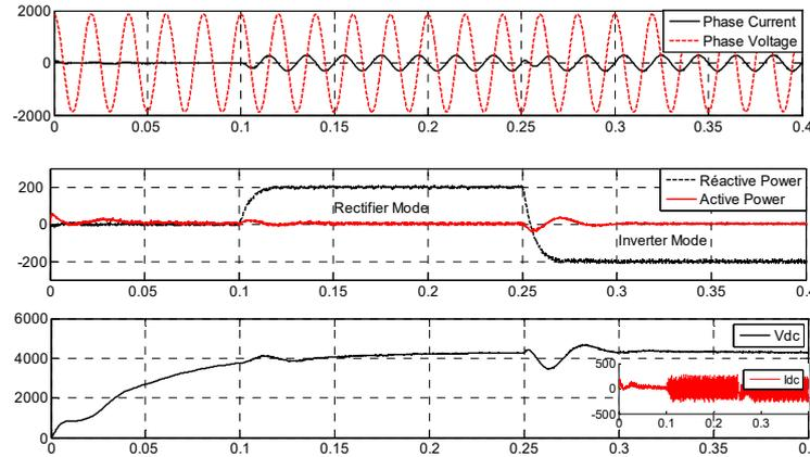
Figure 7.a) Phase Current [Amps], Phase Voltage [volts], b) Active And Reactive Power [watts], c) DC Link Voltage [volts], d) DC Current [Amps].
