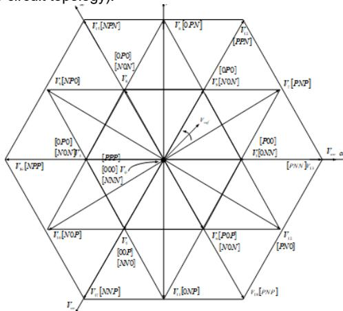
Fig. 2. Space-vector diagram for three-level inverter.
