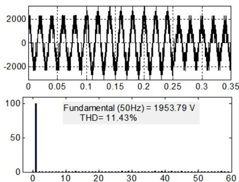
Figure 9 .a) Inverter output voltage [volts], b) Harmonic content from the first phase of the compensator
