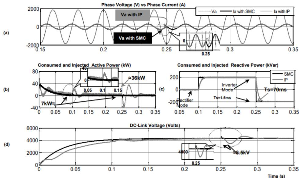
Figure 10 . a) Phase Current [Amps] & Phase Voltage [Volts], b) Active Power [Watts], c) Reactive Power [kVar], d) DC Link Voltage [Volts].
