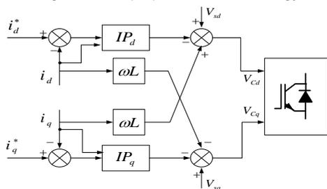
Fig.5. Decoupled Controller.
