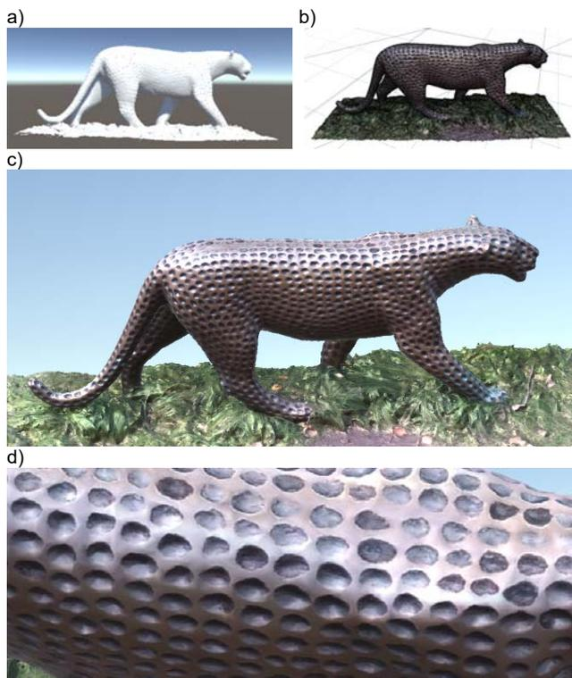
Fig.5. a) solid 3D model b) Wireframe 3D model with material texture c) representation of the 3D model with the texture in VR d) detail of material texture
