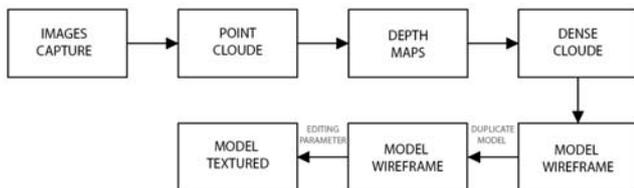
Fig.2. Process of creating 3D models to generate an object texture
