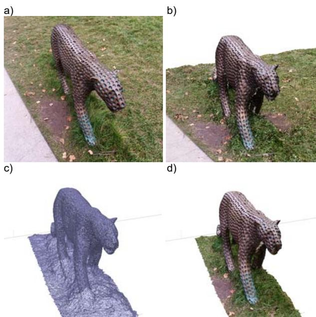
Fig. 1. a) Object photography for 3D modelling b) 3D model of the object in the form of a dense cloud c) Polygonal network 3D model Wireframe d) Basic texture of the 3D model
