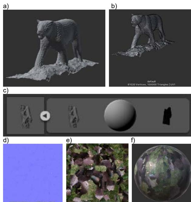
Fig.4. Process of processing 3D models in SW Unity: a) solid shadow 3D model b) Wireframe 3D model c) Content of 3D solid model components d) 2D component texture e) 2D component material f) assembly of components a) and e) in the form of material applied to 3D solid model
