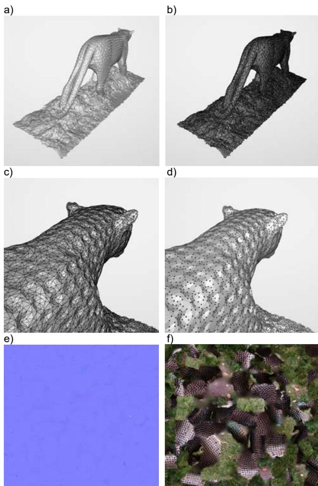
Fig.3. Export of 3D models for application to VR environment: a) solid 3D model generated on the basis of polygonal network and points b) 3D model Wireframe c) detail of 3D model Wireframe d) detail of 3D model in points e) component of exported texture for fixed 3D model f) exported texture component in color attributes for application to a solid 3D model
