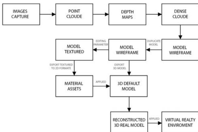
Fig.6. The process of image processing of the material structure of a 3D reconstructed bronze sculpture for application in a VR environment
