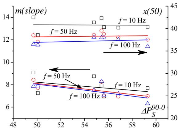
Fig. 5. Parameters  $m$  and  $x(50)$  of Eq. (4) as a function of specific total loss anisotropy  $\Delta P_S^{90-0}$  and frequency  $f$
