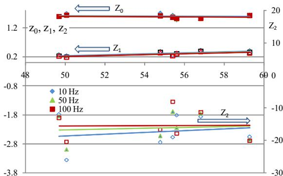
Fig. 6. Parameters  $z_0$ ,  $z_1$  and  $z_2$  of (5) as a function of anisotropy  $\Delta P_S^{90-0}$  and frequency
