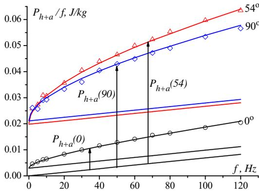
Fig. 1. Energy loss per unit mass versus frequency for different magnetizing directions obtained for steel grade M150-35S at  $B_p = 1.2$  T
