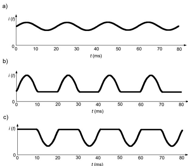
Fig.1. Simplified earth fault current waveforms  $i(t)$  in case of the earth fault on the DC side in a PV installation; according to [12]. Waveforms containing: a) sinusoidal component and smooth DC, b) pulsating DC (half-wave) and smooth DC (both components of the same polarity), c) pulsating DC (half-wave) and smooth DC (components with opposite polarity)
