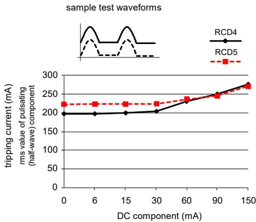
Fig.4. The tripping current of two A-type RCDs of  $I_{\Delta n} = 300$  mA (RCD4, RCD5) under the residual test current composed of: a) AC sinusoidal and smooth DC components, b) pulsating (half-wave) and smooth DC components. The smooth DC component has the following values: 0, 6, 15, 30, 60, 90, 150 mA
