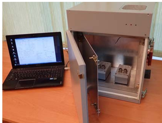
Fig.4. Constant temperature chamber with two resistance standards inside
