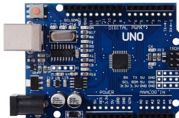
Fig. 3. The Arduino Uno microcontroller used in the aquarium controller model [5].
