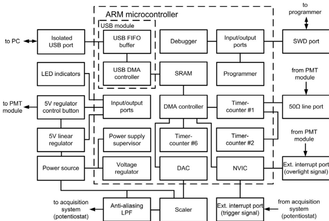
Fig.1. Block diagram of "Pulsar" apparatus.
