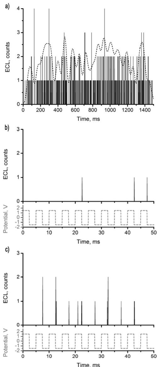
Fig.5. ECL response of ultramicroelectrode for 5ms pulse cyclic polarization: a) general ECL kinetics in millisecond time domain (dotted line is smoothed and  $\times 100$  times magnified ECL counting response), b) first 50 ms of ECL experiment, c) period between 300 ms and 350 ms. The solid line bar is ECL response counts, the dash line is the electrode polarization potential.
