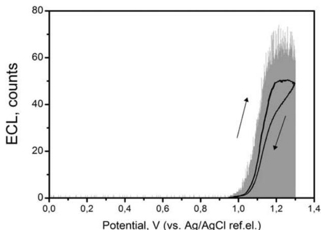
Fig.4. ECL response for  $\text{Ru}(\text{bpy})_3^{2+}$  + TPA composition. The black curve is the analog signal representation with 1 ms resolution (arrows show direction of signal with a potential scan). The grey curve is the digital signal representation with 10  $\mu$ s resolution.
