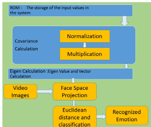
Fig 4: Hardware Implementation of Emotional Recognition
