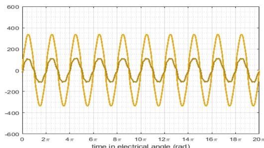
Fig. 14. Voltage and current waveforms in supply line R of the compensated load.
