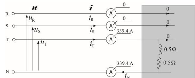
Fig. 2. An example of an unbalanced load.
