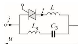
Fig. 7. A TCS branch built of TSI branch and a filter of the 3<sup>rd</sup> order harmonic.
