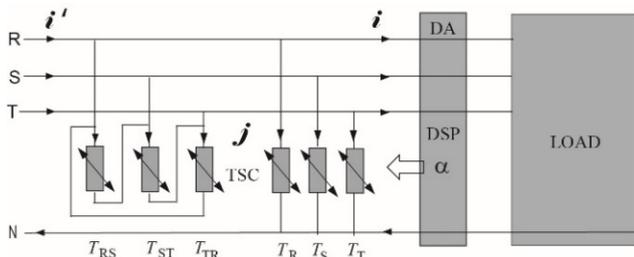
Fig. 9. A structure of an adaptive compensator.
