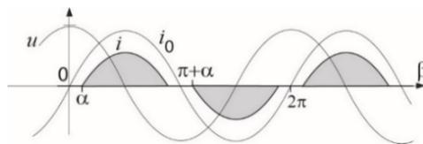
Fig. 5. The currents waveform of a thyristor switched inductor (TSI).
