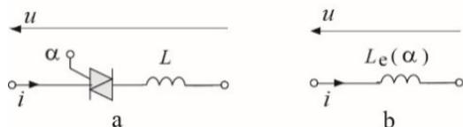
Fig. 4. A thyristor switched inductor (TSI) (a) and its equivalent inductance (b).
