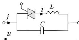
Fig. 1. A thyristor-switched inductor with a shunt capacitor.
