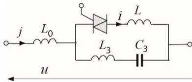
Fig. 8. A TSC branch with 3<sup>rd</sup> harmonic filter and series inductor  $L_0$ .
