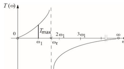
Fig. 11. Change of the TCS branch in the thyristor OFF state.
