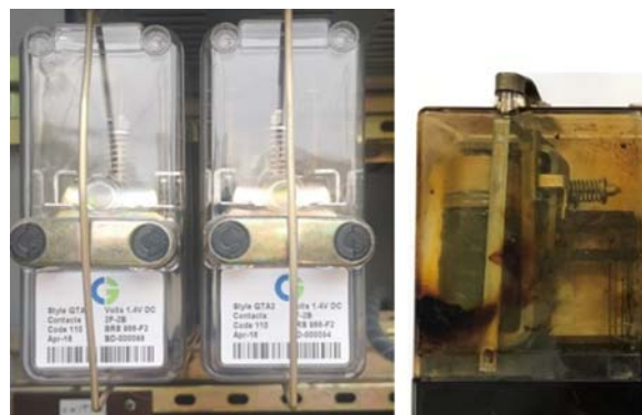
Fig. 7. Installation and burning of the BR966F2 relay from overvoltage.
