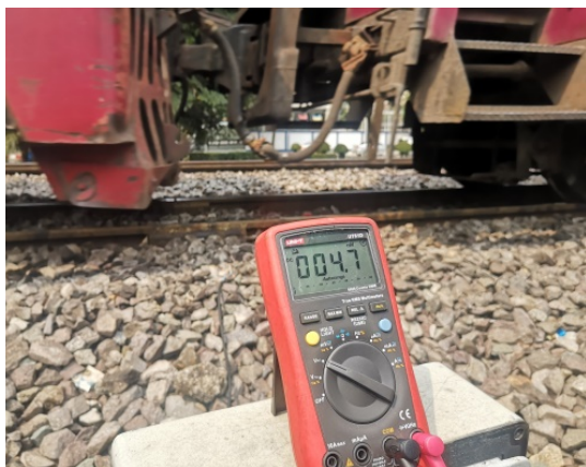
Fig. 4. Voltage drop 4.7 mV while there is a train.
