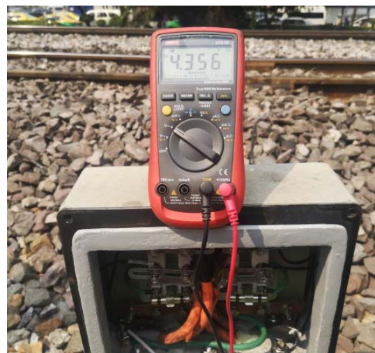
Fig. 3. Voltage drop on the track 4.356V while the track is clear.
