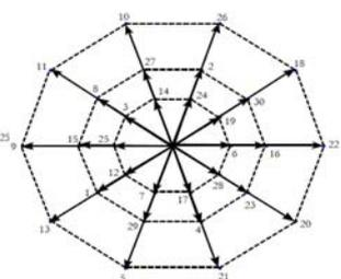
Fig.2. Projection of voltage vectors in the main plan Fig.3. Projection of voltage vectors in the secondary plan
