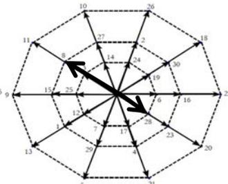
Fig.4.b. Representation of the active vectors in both plan secondary
