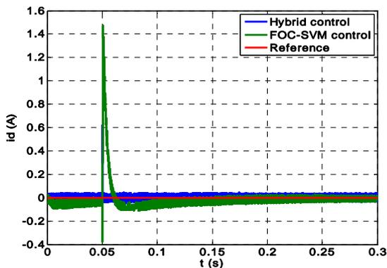
Fig.10. Current  $i_d$  for both controls
