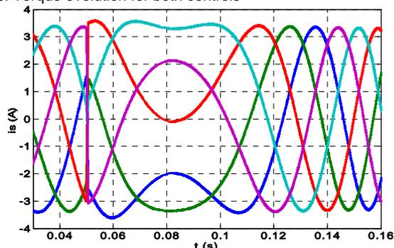
Fig.9. Currents of phases in the case of FOC-SVM
