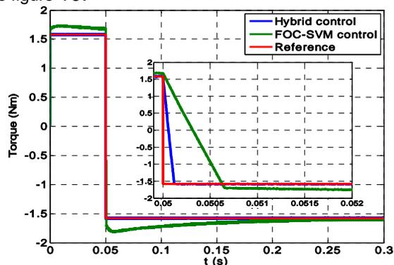
Fig.8. Torque evolution for both controls
