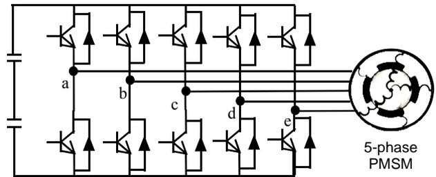
Fig.1. Example of a five-phase inverter for the five-phase synchronous machine.
