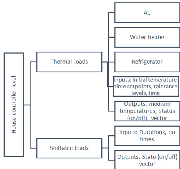
Fig.2. Structure of the complete house controller model
