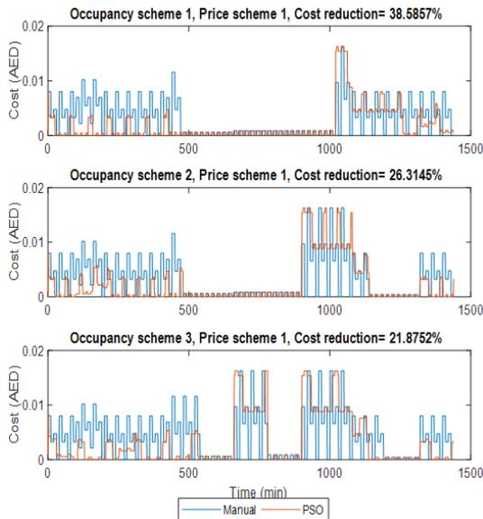
Fig. 8. Manual (baseline) controller cost vs PSO cost
