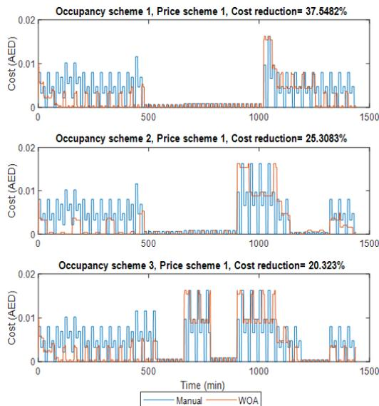
Fig. 9. Manual (baseline) controller cost vs WOA cost
