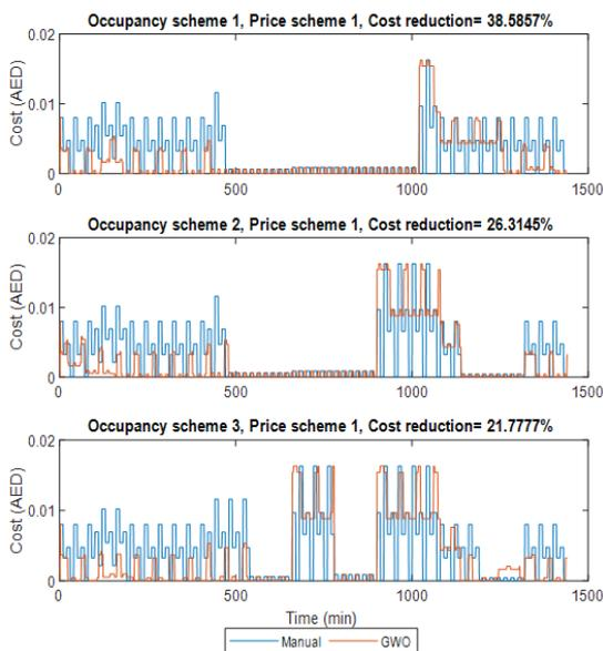
Fig. 10. Manual (baseline) controller cost vs GWO cost
