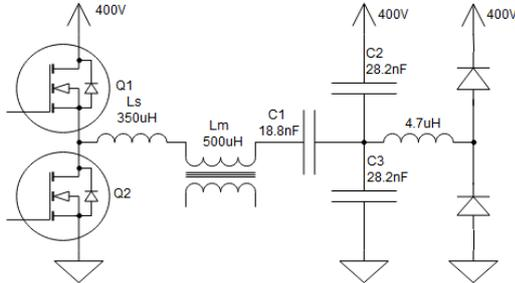
Fig.1. Overview of the components in the LLC resonant converter with quality factor limiter [5]
