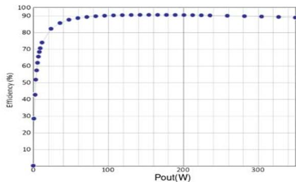
Fig. 10. Measured converter efficiency.
