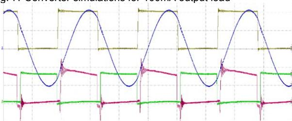
Fig. 8. Converter measurements for 30 A output load (5 us/div). Yellow: half-bridge voltage (200 V/div), blue: Ls current (2 A/div); pink and green: half-bridge driving signals (2 V/div).
