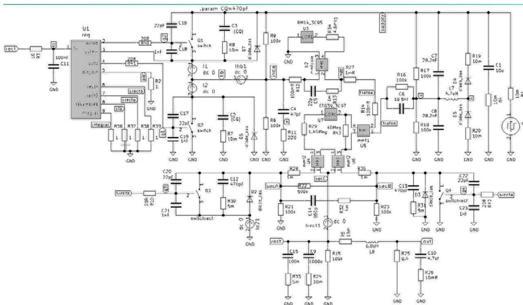
Fig.2. Schematic of the simulated system with measured values of inductances and parasitic elements of real LLC resonant circuit.
