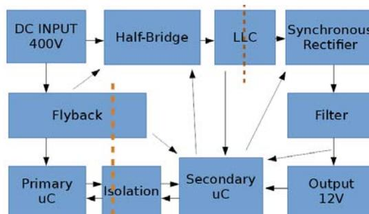
Fig. 4. Physical model block diagram
