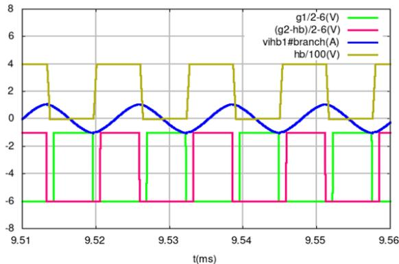
Fig. 7. Converter simulations for 100mA output load
