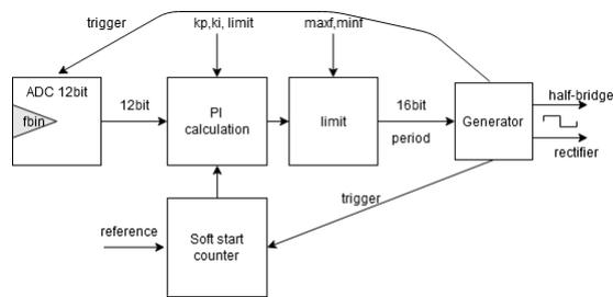
Fig. 3. Output voltage controller block diagram
