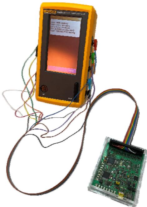
Fig.3. Our FLUKE model ProSim 4 ECG simulator with our own hardware for collecting real ECG data.
