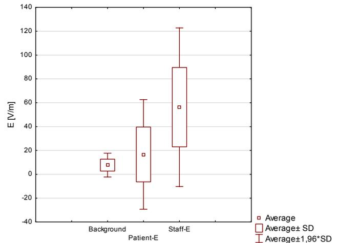
Fig. 8 Box plot for the measurement of the electrical component of the device – mean/standard deviation
