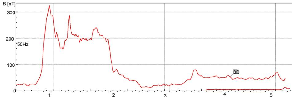
Fig. 5: Measurement of the electromagnetic field during operation of the device, a) electric component E,(V/m), b) magnetic induction B, (nT)
