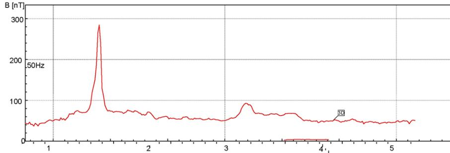
Fig. 4. Measurement of the background electromagnetic field of the surgery, a) electric component E,(V/m), b) magnetic induction B, (nT)
