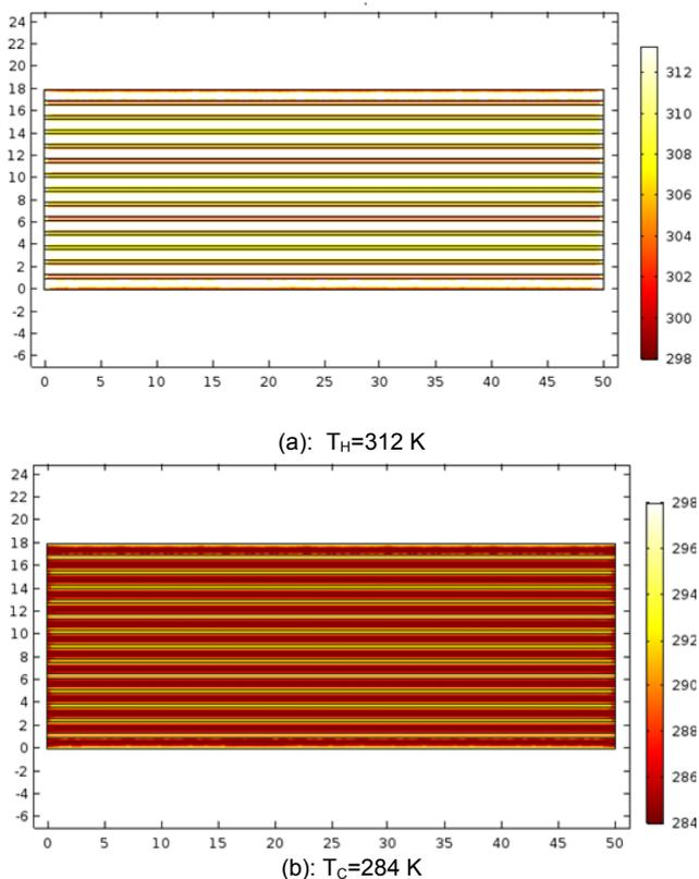
Fig.5. Temperature distribution during: The hot blow (a); and the cold blow (b) for Al<sub>2</sub>O<sub>3</sub>
