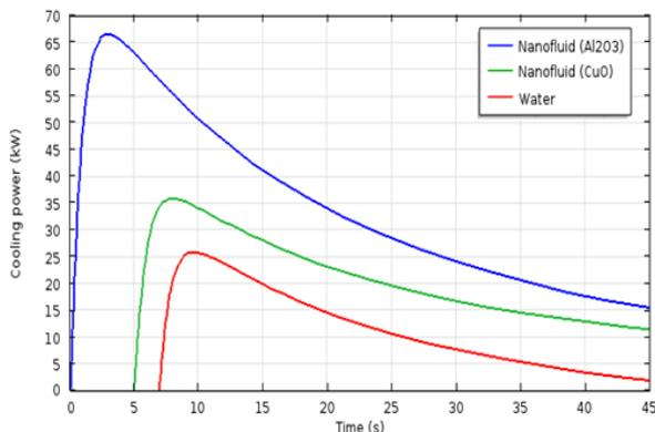
Fig.7.The variation of cooling capacity as a function of time
