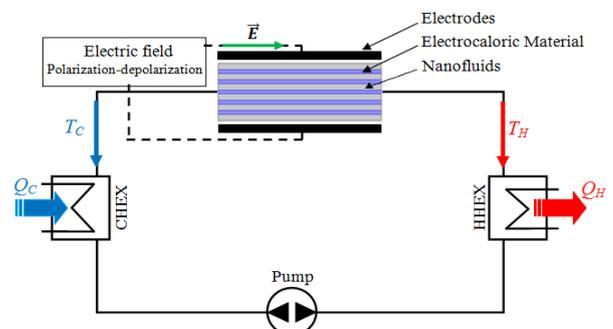
Fig. 1. Schematic diagram of the AER cycle setup
