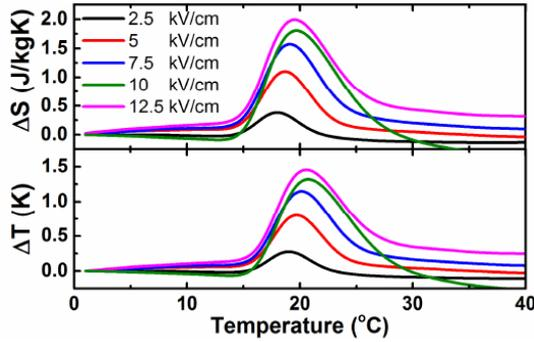
Fig.2. Electrocaloric effect in BaTiO3 ceramics near room temperature [6]
