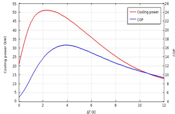
Fig.8.The variation of cooling capacity and coefficient of performance (COP) for  $Al_2O_3$  as a function of temperature difference
