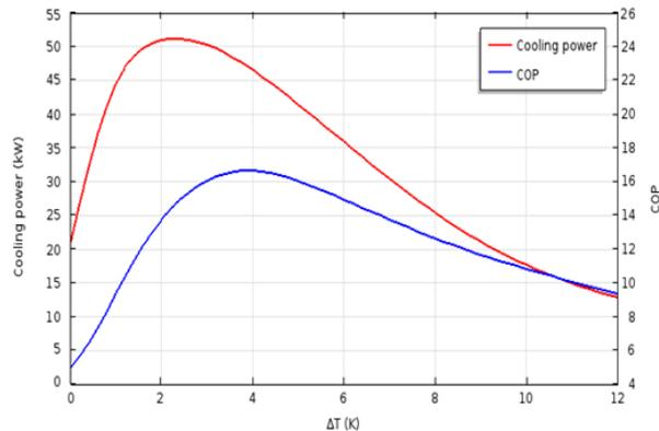
Fig.8.The variation of cooling capacity and coefficient of performance (COP) for  $Al_2O_3$  as a function of temperature difference
