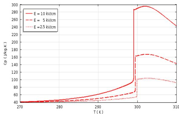
Fig.10.The variation of heat capacity as a function of temperature
