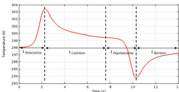
Fig.4. The evolution of the regenerator temperature during a cycle
