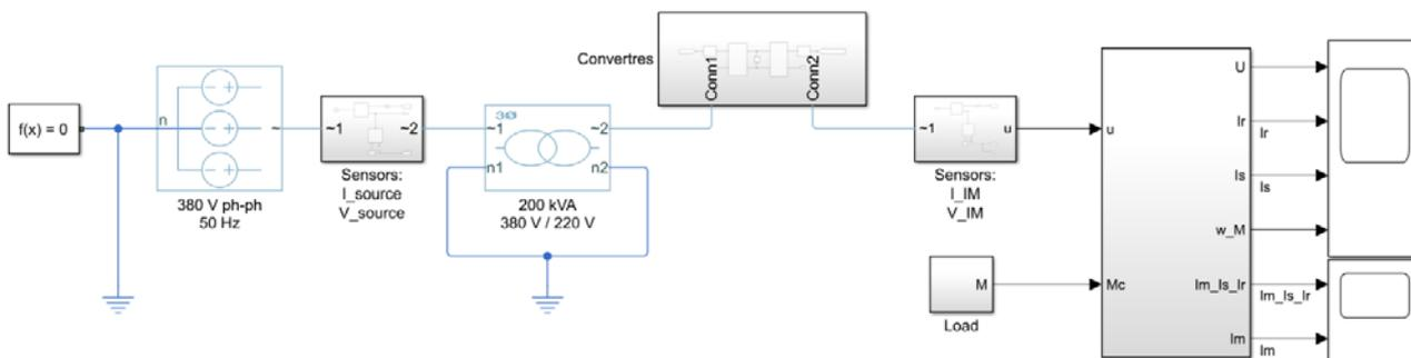
Fig. 3. Simulation model for electric drive control system
