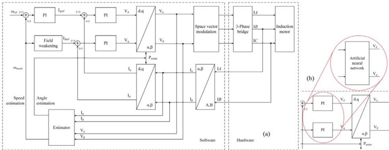
Fig. 1. Induction motor FOC control: a – traditional scheme; b – replaced blocks
