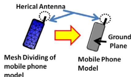
Fig.2. Mobile Phone model with the helical antenna and ground plane.
