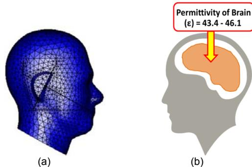
Fig.1. (a) Flat SAM; Model A. (b) The brain inserted into the flat SAM; Model B
