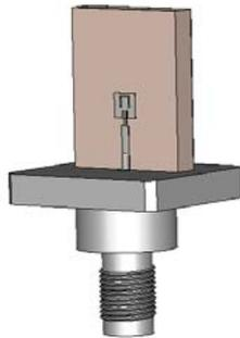
Fig.4. 5G 60-GHz antenna for the VR headset.
