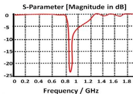
Fig.3. Simulation of the S-Parameter of the IEEE Mobile Phone 900 MHz (effective frequency of the monopole helical antenna).
