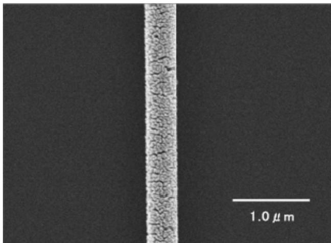
Fig.5. Photograph of FE-SEM image of silver pipe.
