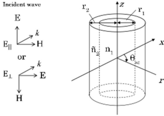
Fig.1. Schematic diagram of Ag pipe and coordinate axes.
