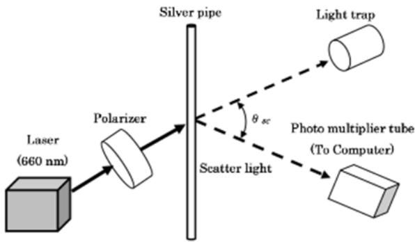
Fig.2. Experimental setup of measuring devices.
