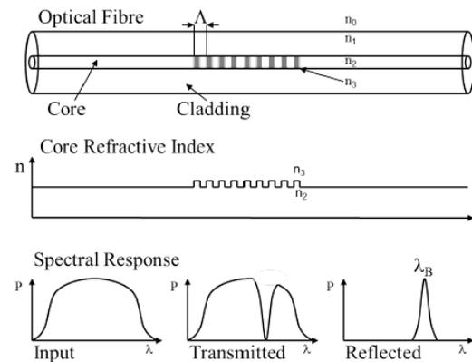
Fig.1. The principle of operation of FBG
