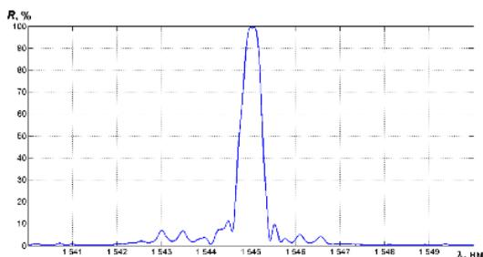
Fig. 4. The reflection spectrum of the apodized Bragg grating
