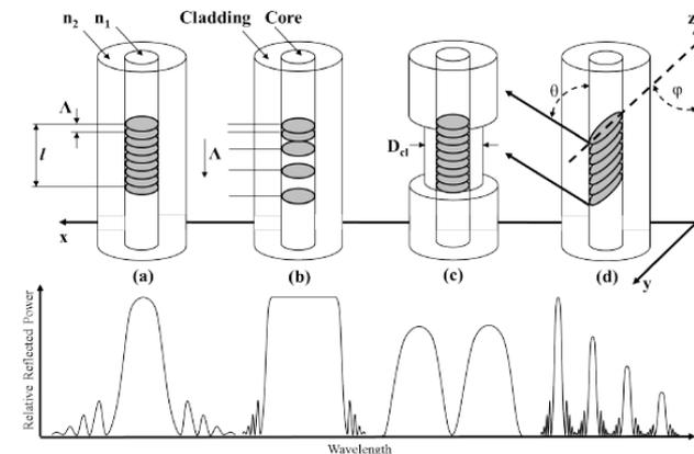
Fig.2. Various types of gratings and their spectral characteristics
