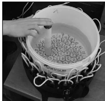
Fig. 1 The test stand with 32 transducers arranged around the bucket
