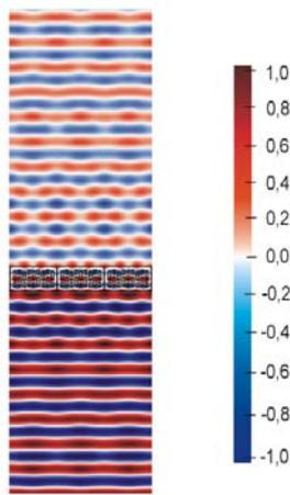
Fig.2. The 2D distribution of relative value of  $E_z$  component inside analysed area with the wall made of bricks ( $s=0.011$  m)
