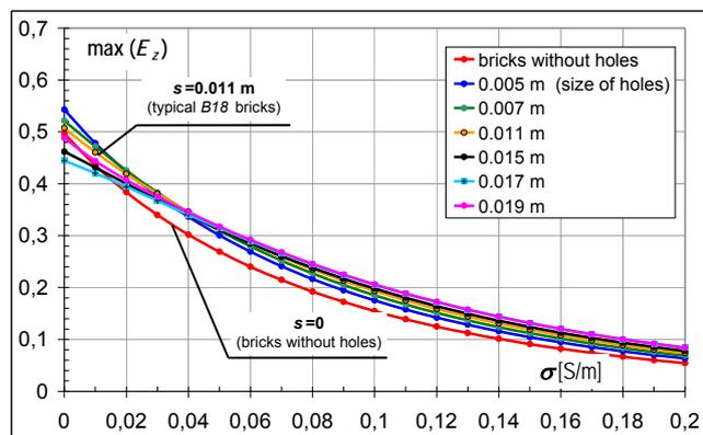
Fig.3. The relative maximum values of  $E_z$  component behind the analysed wall made of bricks with different size of holes
