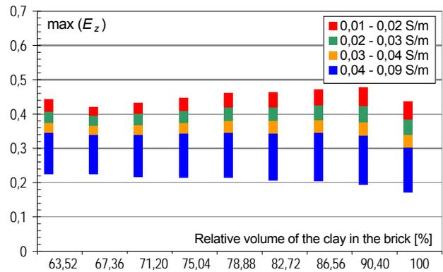
Fig.4. The dependence between  $\max(E_z)$  and the relative volume of the clay inside the brick
