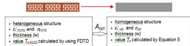
Fig.5. Task scheme and connection of input and output data in the implementation of the developed numerical algorithm ( $A_{opt}$ )
