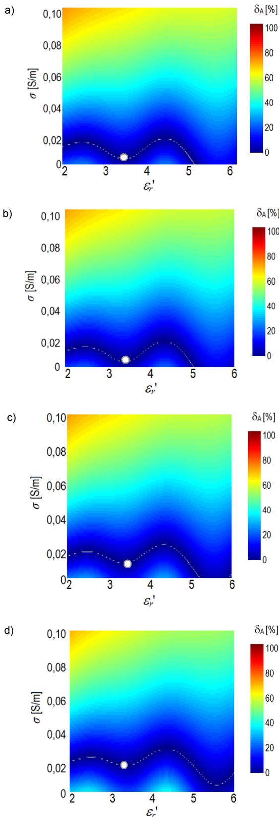
Fig.7. Calculated substitute relationship between relative electric permittivity and conductivity in a model with a wall made of hollow bricks, with the initial assumption: a)  $\sigma_{\text{FDTD}}=0.01$  S/m, b)  $\sigma_{\text{FDTD}}=0.02$  S/m, c)  $\sigma_{\text{FDTD}}=0.03$  S/m, d)  $\sigma_{\text{FDTD}}=0.04$  S/m
