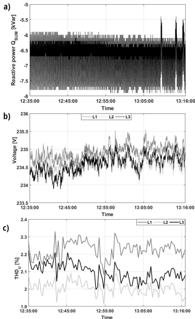
Fig. 9. Test 2 – Measurements of reactive power (a), phase voltage (b) and THD<sub>U</sub> (c)
