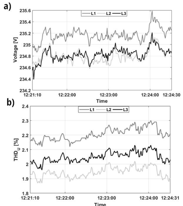
Fig. 7. Test 0 – Measurements of phase voltage (a) and  $THD_U$  (b)
