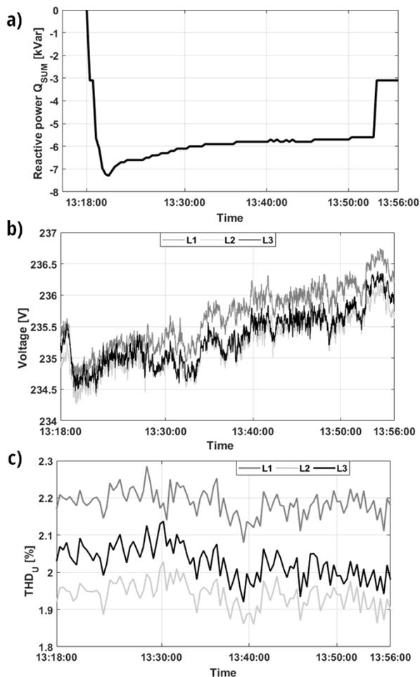
Fig. 11. Test 4 – Measurements of reactive power (a), phase voltage (b) and  $THD_U$  (c)
