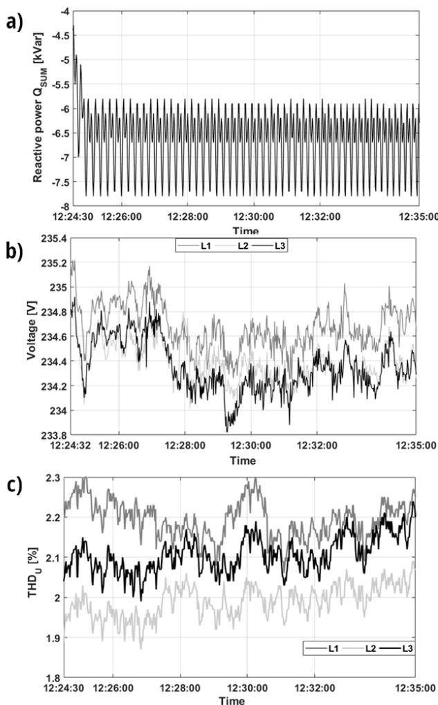
Fig. 8. Test 1 – Measurements of reactive power (a), phase voltage (b) and THD<sub>U</sub> (c)
