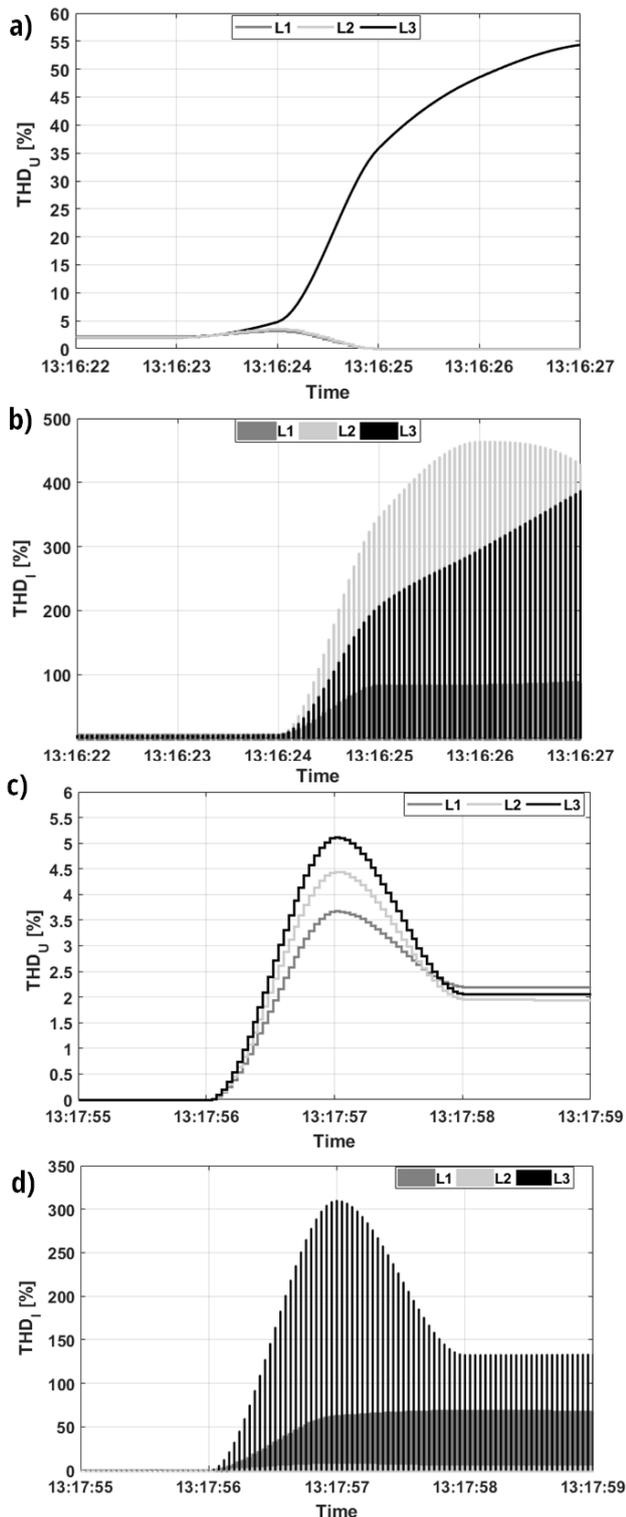
Fig. 10. Test 3 – Measurements of  $THD_U$  during switch off (a),  $THD_I$  during switch off (b),  $THD_U$  during switch on (c) and  $THD_I$  during switch on (d)
