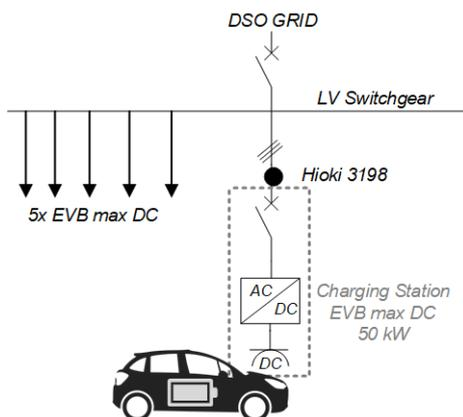
Fig. 5. Single line diagram of LV substation at Orzeszkowa Street
