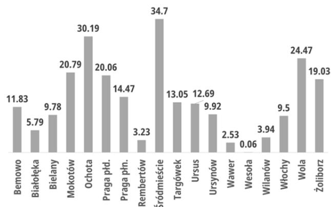
Fig. 3. The degree of MV network cabling in Warsaw area – length of cable lines [km] per 1 km<sup>2</sup> of district area
