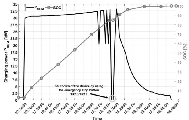
Fig. 6. Measurements of charging power and SOC of EV during whole test
