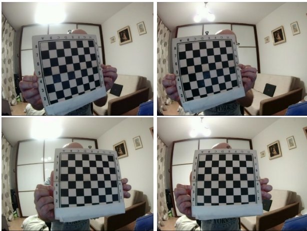
Fig 1. This figure presents example pairs of pictures with the chessboard that we used for camera calibration. The complete set of calibration pictures is available in digital repository [22].
