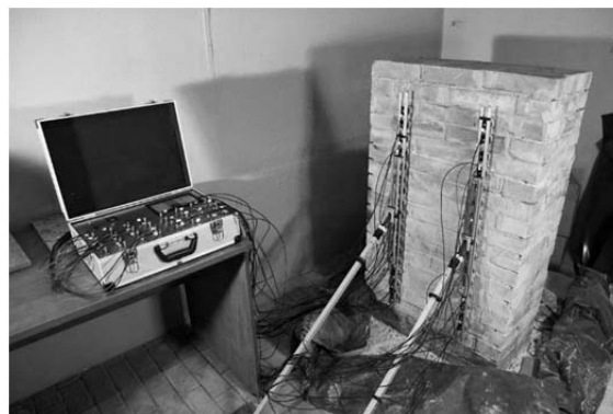
Fig. 10. Hybrid tomograph 2.0 to use the tomograph to measure the test wall.
