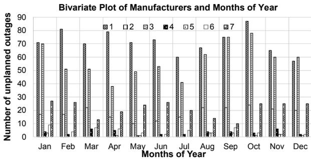
Fig. 21: Bivariate bar chart of number of forced outages for various manufacturers against the number of forced outages for months of the year.
