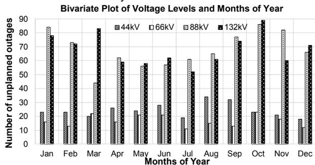
Fig.17: Bivariate bar chart of number of forced outages for various kVs against the number of forced outages for various months of the year.
