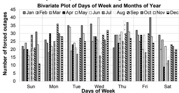
Fig. 28: Bivariate bar chart of number of forced outages for various months of the year against the number of forced outages for various days of the week.
