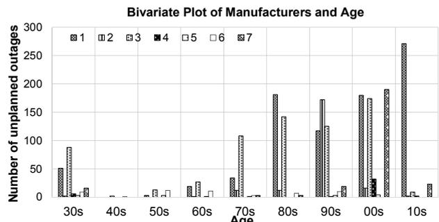
Fig. 20: Bivariate bar chart of number of forced outages for various manufacturers against the number of forced outages for various ages.
