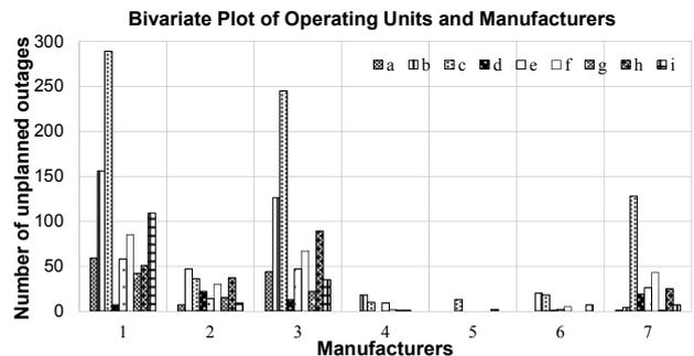
Fig. 9: Bivariate bar chart of number of forced outages for various OUs against the number of forced outages for various manufacturers.
