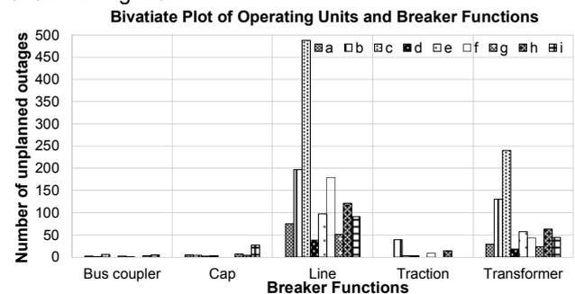
Fig. 10: Bivariate bar chart of number of forced outages for various OUs against the number of forced outages for various breaker functions.
