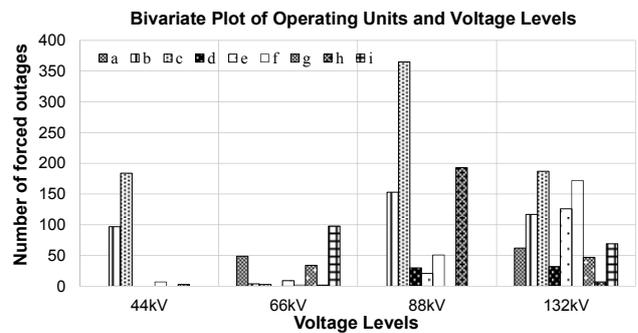
Fig. 8: Bivariate bar chart of number of forced outages for various OUs against the number of forced outages for various kV levels.
