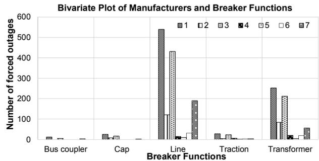
Fig.19: Bivariate bar chart of number of forced outages for various manufacturers against the number of forced outages for various breaker functions.
