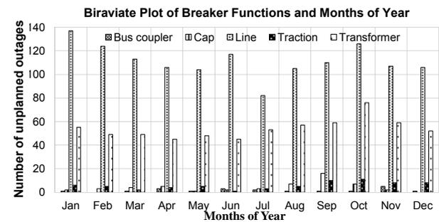
Fig. 24: Bivariate bar chart of number of forced outages for various breaker functions against the number of forced outages for various months of the year.
