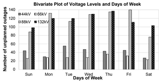
Fig. 18: Bivariate bar chart of number of forced outages for various kVs against the number of forced outages for various days of the week.
