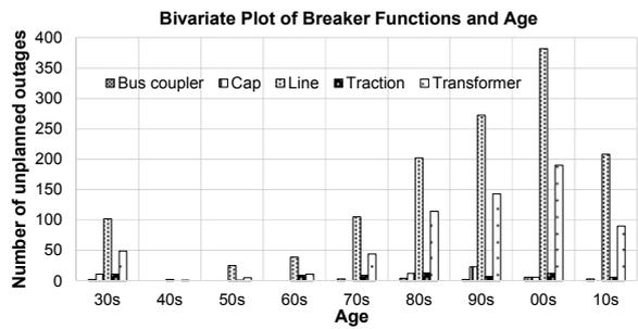
Fig. 23: Bivariate bar chart of number of forced outages for various breaker functions against the number of forced outages for various ages.
