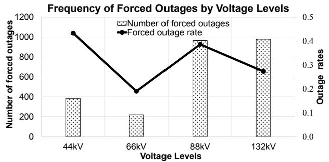
Fig. 2: Frequency of forced outages for various voltage levels.
