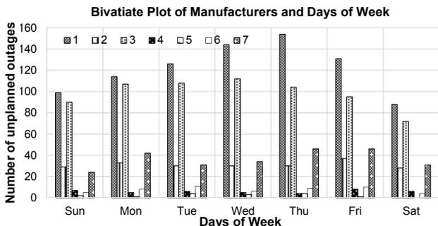
Fig. 22: Bivariate bar chart of number of forced outages for various manufacturers against the number of forced outages for various days of the week.
