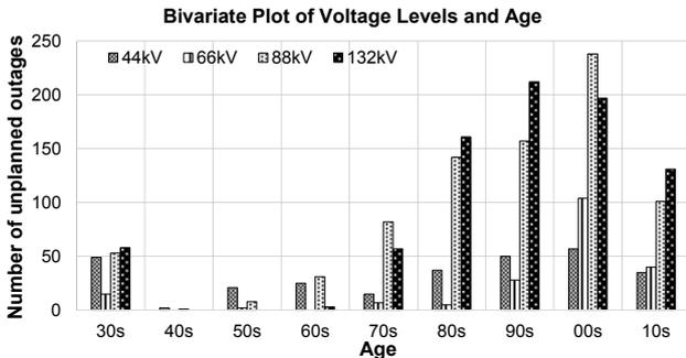
Fig. 16: Bivariate bar chart of number of forced outages for various kVs against the number of forced outages for various ages.
