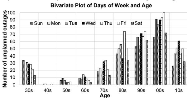
Fig. 27: Bivariate bar chart of number of forced outages for various days of the week against the number of forced outages for various ages.
