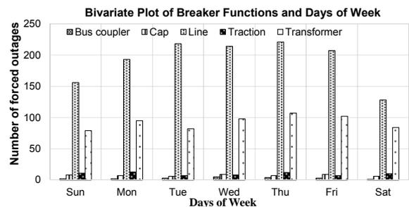
Fig. 25: Bivariate bar chart of number of forced outages for various breaker functions against the number of forced outages for various days of the week.
