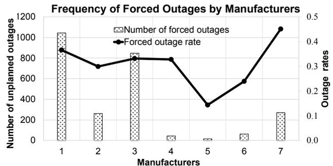
Fig. 3: Frequency of forced outages for various manufacturers.
