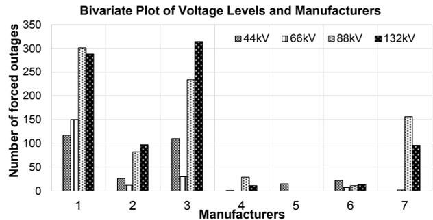
Fig.14: Bivariate bar chart of number of forced outages for various kVs against the number of forced outages for various manufactures.
