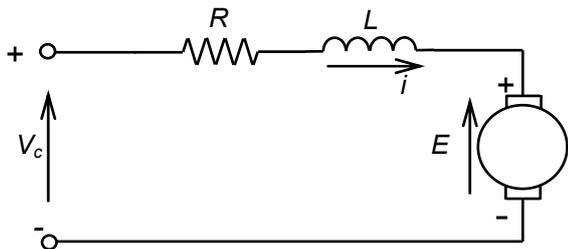
Fig. 2. Schematic of Permanent Magnet DC motor
