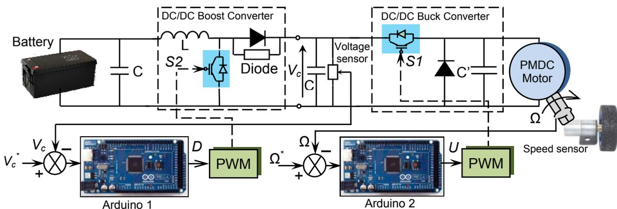
Fig. 3. Battery and DC/DC converters for electric vehicle control
