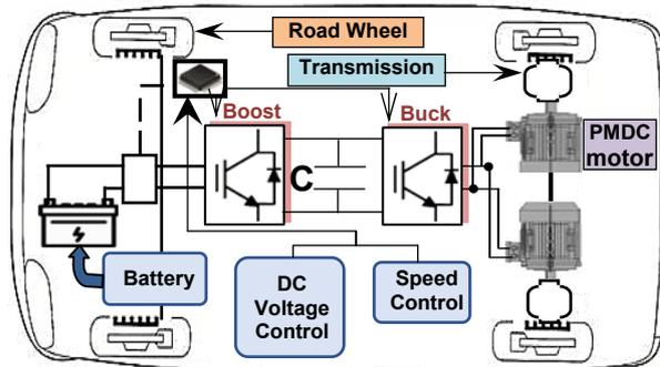
Fig. 1. Main components of the proposed EV
