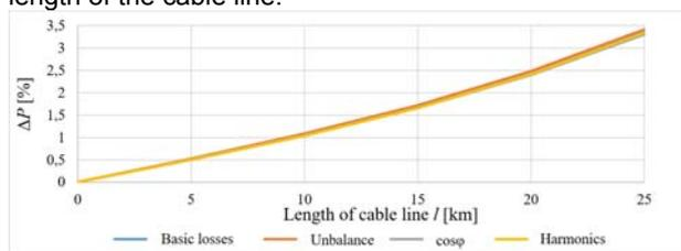
Fig.17. Active power losses on MV side for Location 6
