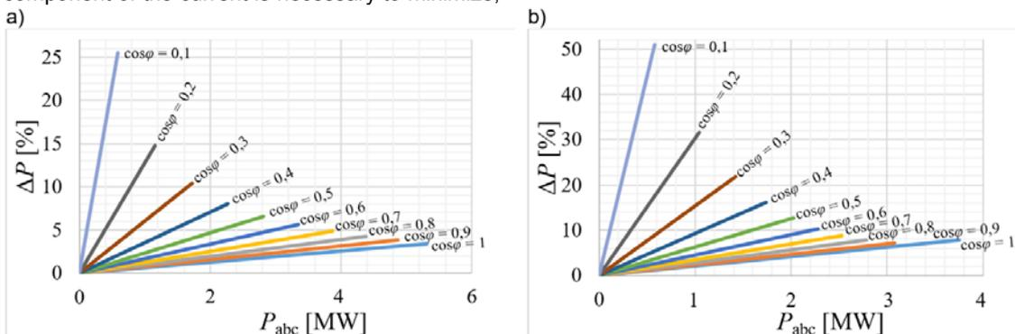
Fig. 10. The active power losses for NA2XS2Y 95/16: a) the length of 10 km, b) the length of 30 km
