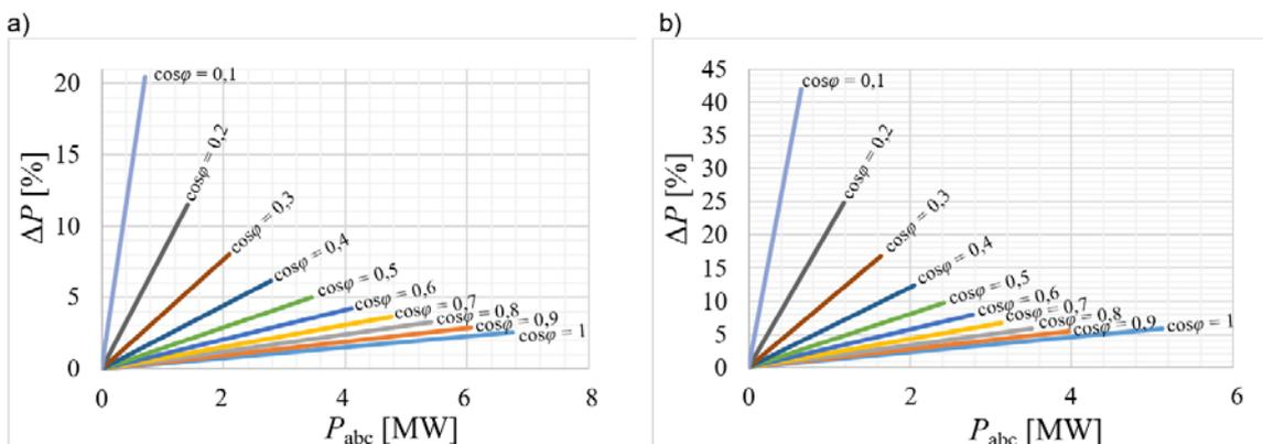
Fig. 11. The active power losses for NA2XS2Y 150/25: a) the length of 10 km, b) the length of 30 km
