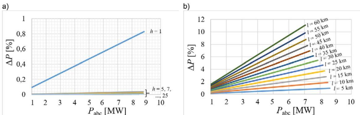
Fig. 15. The active power losses for NA2XS2Y 240/25: a) the length of 5 km, b) the different length
