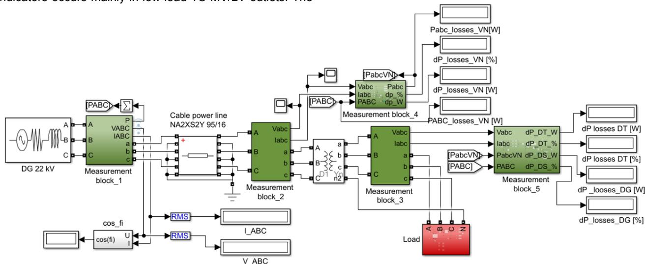
Fig.16. Simulation model of distribution grid
