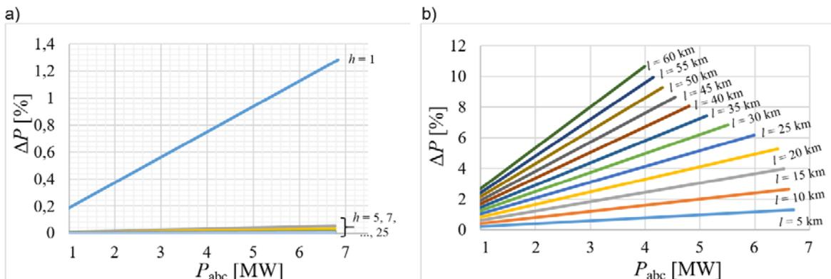
Fig. 14. The active power losses for NA2XS2Y 150/25: a) the length of 5 km, b) the different length
