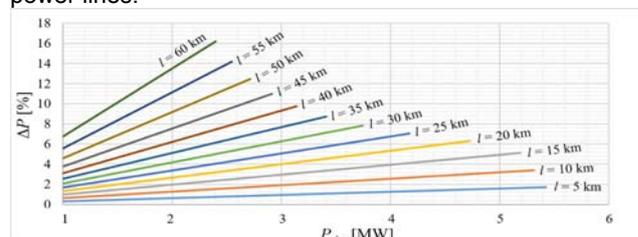
Fig.1. The active power losses for NA2XS2Y 95/16
