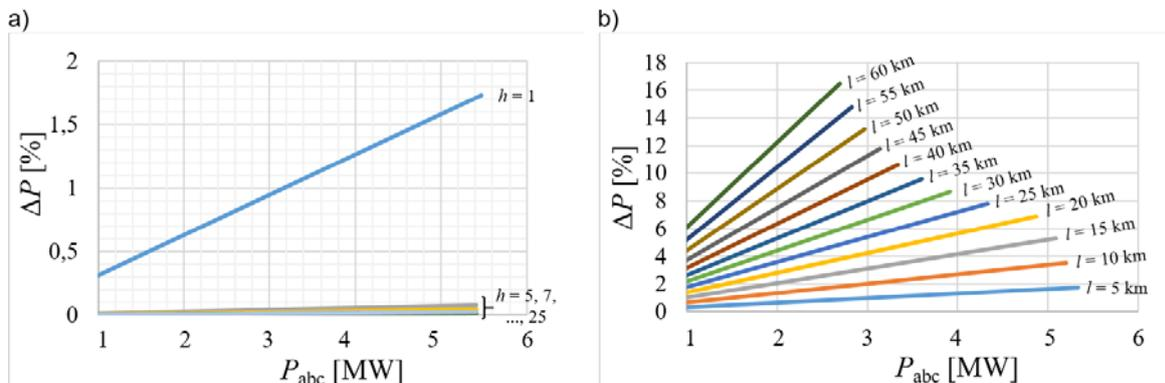
Fig. 13. The active power losses for NA2XS2Y 95/16: a) the length of 5 km, b) the different length
